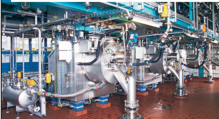
**GMP-compliant filtration centrifuges from ANDRITZ KMPT are qualified for challenging separation processes with minimum product loss in the pharmaceutical industry.**
